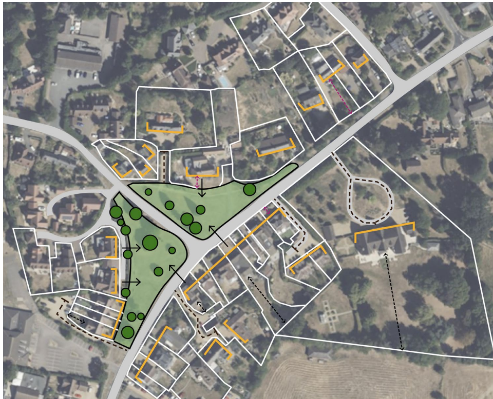
Figure 28: Example of informal development pattern around The Village Green in Bromham, which is part of the older area of the village. There is high variation in plot sizes, shapes and set-back distances, with a significantly larger plot at 86 Village Road. There is also variation in orientation and pattern of development with some linear plots and consistent building line and also examples of long driveways to individual properties and small closes. There are high levels of natural surveillance over The Village Green afforded by the short set-backs of the some of the houses surrounding it. However there are also examples of long front gardens, up to about 36m. Back gardens range from approximately 10 to 80m.
